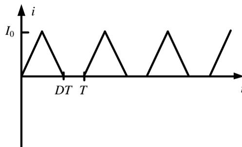
Figure 4. Triangular current waveform.
