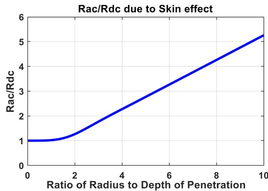
Figure 2.  $R_{ac}/R_{dc}$  due to skin effect.
