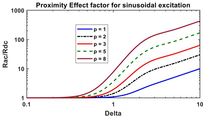
Figure 3. Proximity effect for different number of layers.
