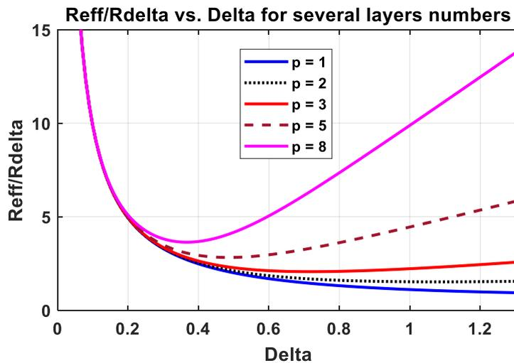
Figure 5. The effective resistance versus the layer thickness for different number of layers.
