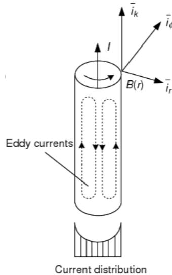
Figure 1. Eddy currents in a round conductor [1].
