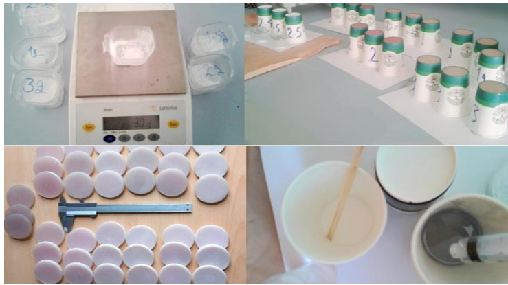
Figure (3): Samples of impure polyester reinforced with pure calcium carbonate and eggshells.
