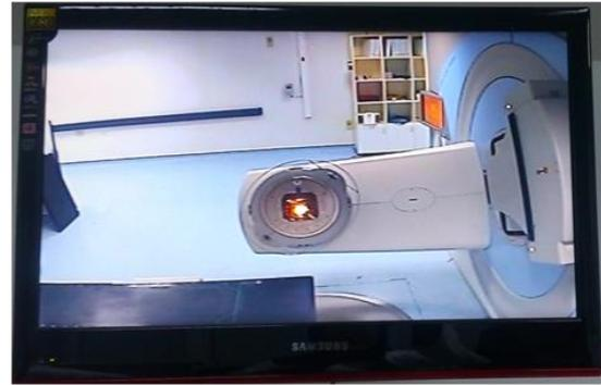
Fig. 2.4: shows the Synergy's gantry position during the radiation survey procedure (taken from the camera), which is the position at which the primary radiation is face to face to the control console.
