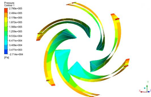
Figure 10:- Cavitation Model on six blades with 16 kg/s mass flow rate.
