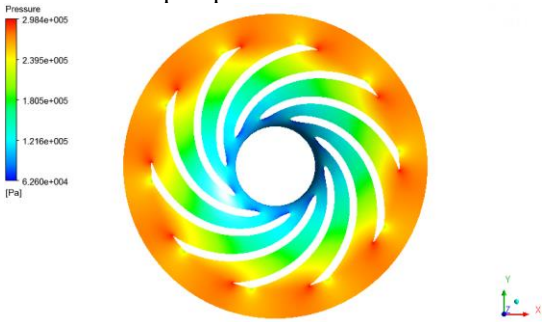
Figure 9:- Pressure Distribution of Centrifugal Pump Impeller with 10 blades
