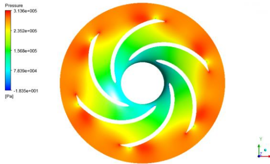
Figure 7:- Pressure Distribution of Centrifugal Pump Impeller with 6 blades
