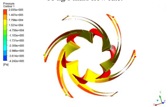
Figure 10:- Cavitation Model on six blades with 16 kg/s mass flow rate.
