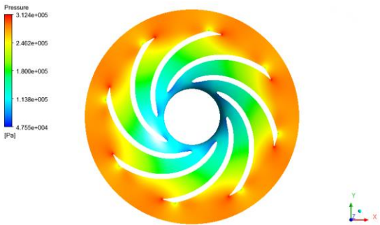
Figure 8:- Pressure Distribution of Centrifugal Pump Impeller with 8 blades
