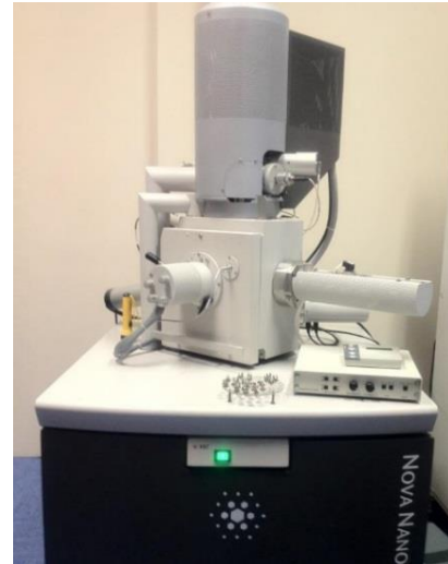
Figure 1: Scanning electron microscopy (SEM) used for determining elemental composition of orthodontic archwires
